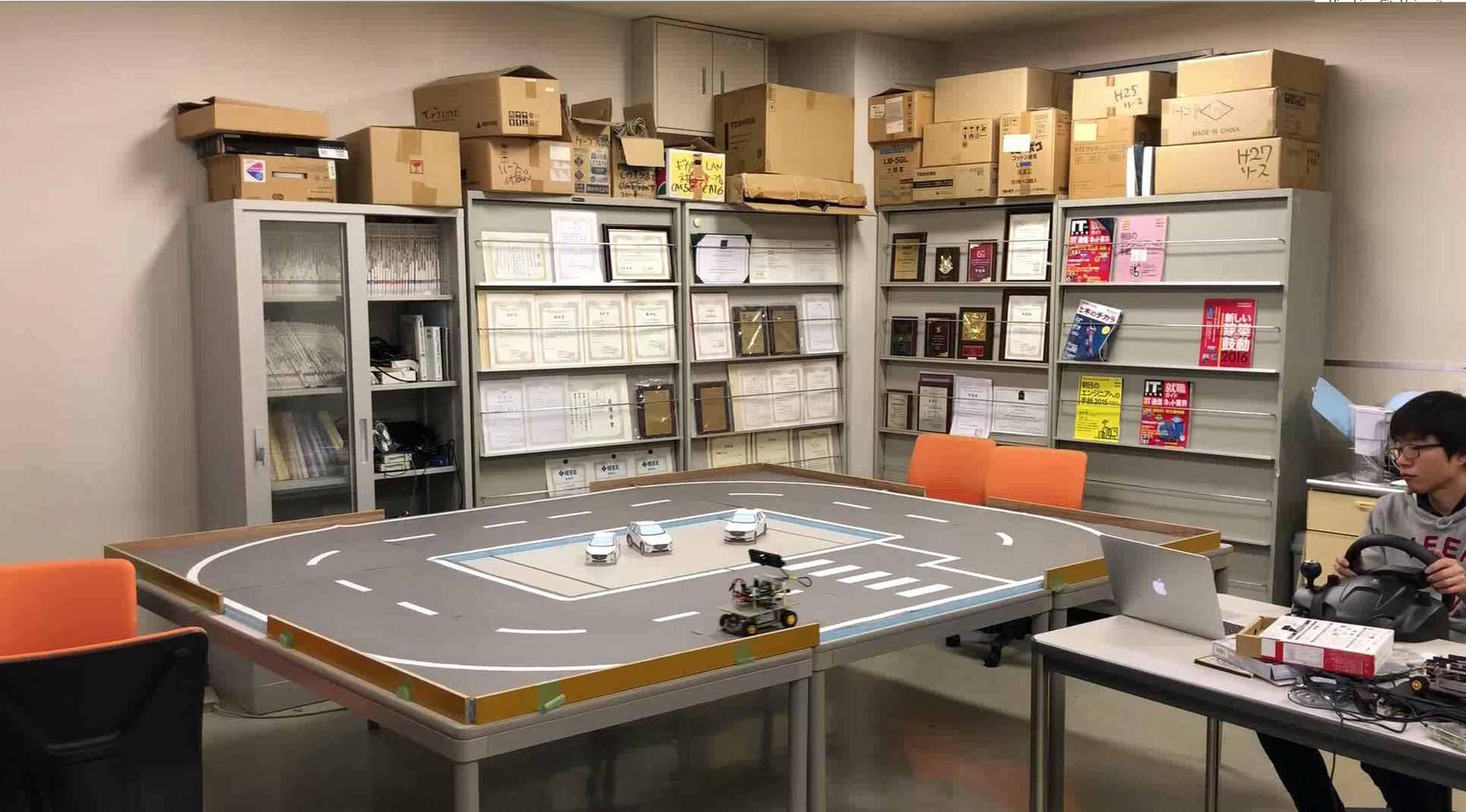
0:00 – 0:29 : Driving the car and training CNN by human steering in real time
